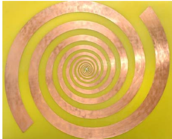
Figure 3. Fabricated log spiral antenna.
